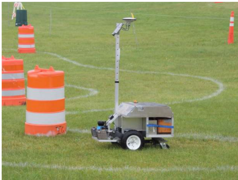
Figure 1: An autonomous vehicle moving within the lane and about to avoid an obstacle during 2013 IGVC [2].
