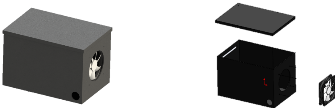
Figure 10: Electronic housing compartment assembly (left) and exploded view (right)
